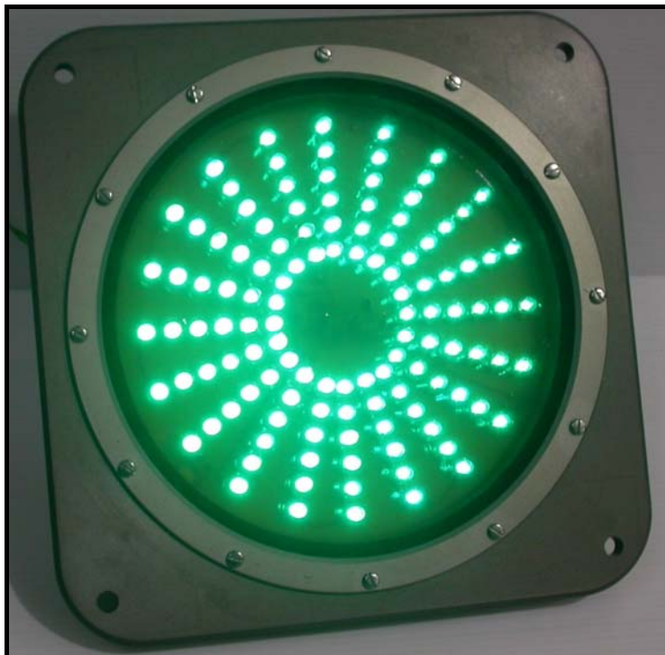
Green Traffic Light Array
